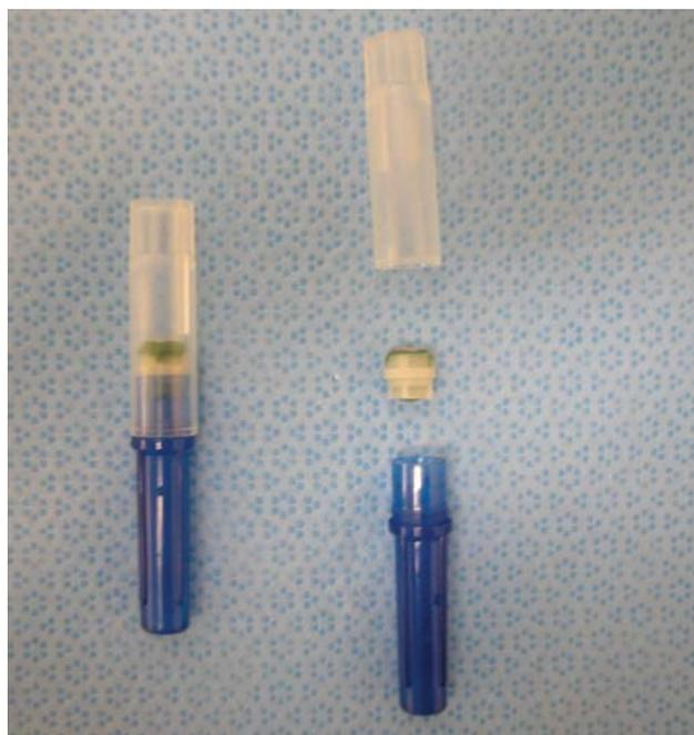
**Figure 2.** Assembled and disassembled dentin cylinder model.
